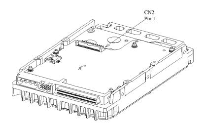
Figure 5.2 IDD setting terminals position (MP model only)
